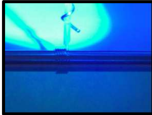
Movie S3. Video of filament deposition on a rotating rod for fabricating hollow tube structures. 2.5 wt% MeHA was used. Video was 12 times faster than realtime.
