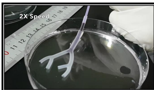
Movie S1. Perfusion demonstration of a quadrifurcate vasculature-like structure. DI water supplemented with food dye was perfused through branched hollow channels using syringe.
