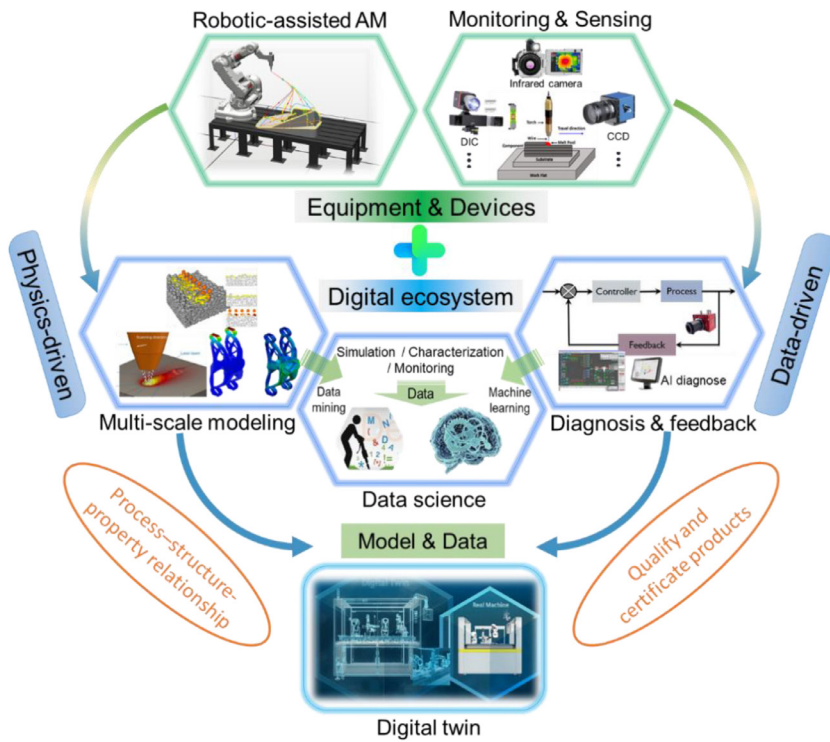
Fig. 6. Schematic illustration of the physics- and data-driven AM framework based on advanced devices and digital ecosystem.
